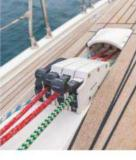
Left: a deck locker for diesel fillers with raised caps to help prevent spillage Right: running rigging (and jib sheets) lead neatly to a bank of high-load jammers aside the cockpit electric motors. Hydraulic winches and furlers also make it easier for one person to control sail operations remotely from
